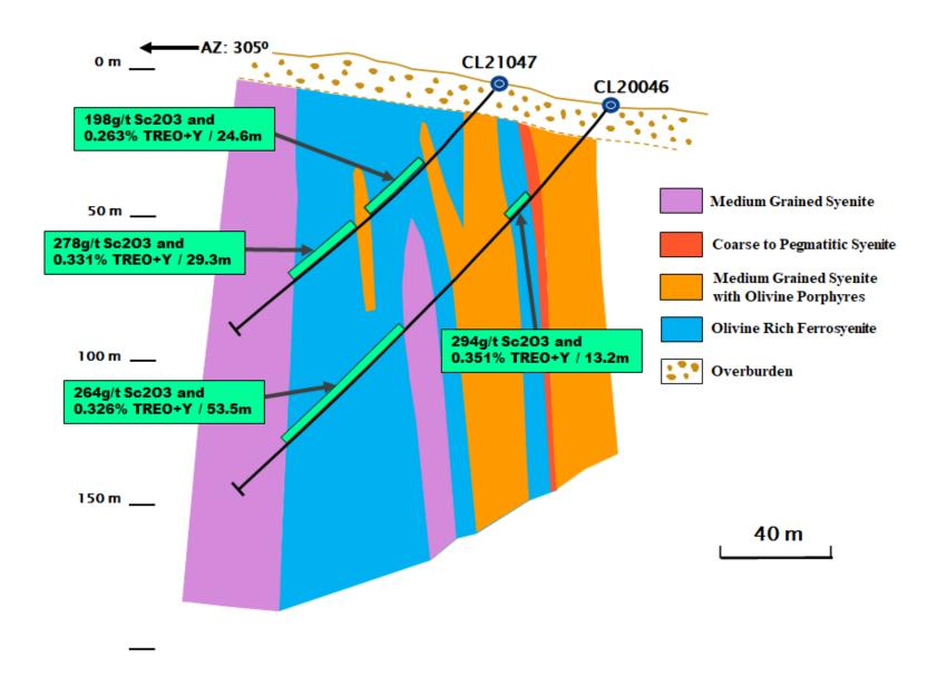
Figure 2 – Diamond Drill Cross-Section 400N, TG Zone, Crater Lake Project, Quebec
